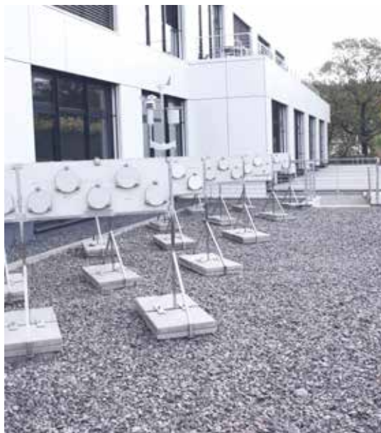
3 Layout of the plaster discs
